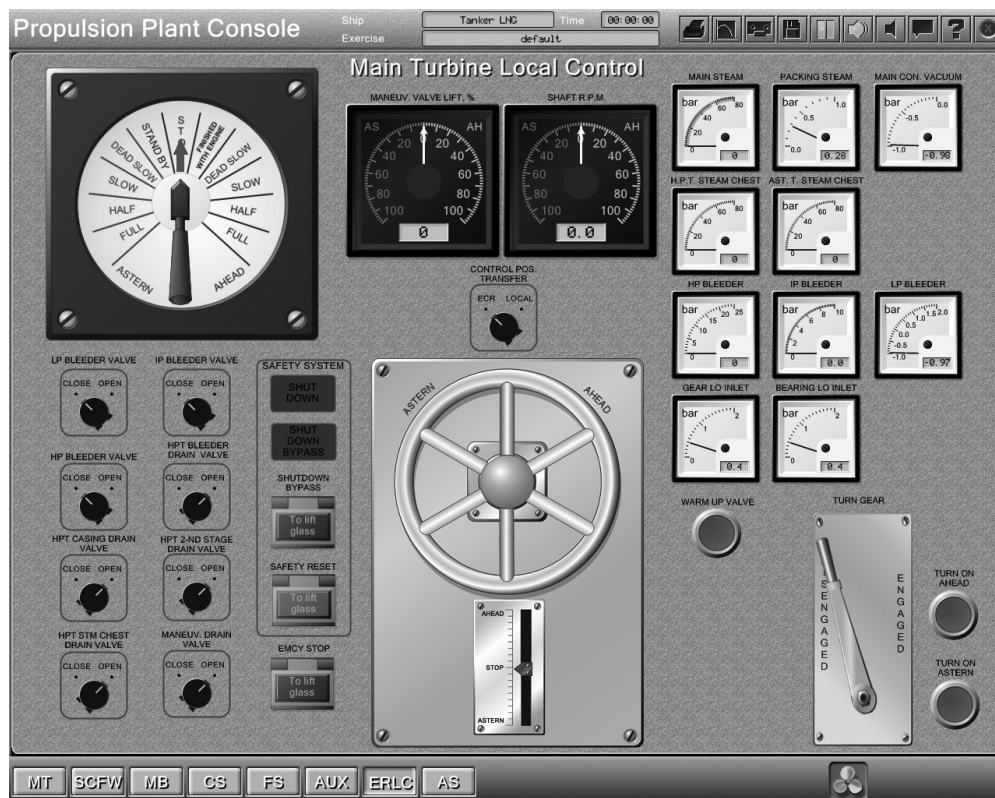
Fig. 23. Main Turbine Local Control panel
